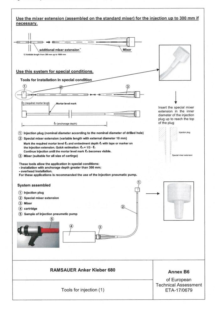
Table B5: Mortar injection pumps
